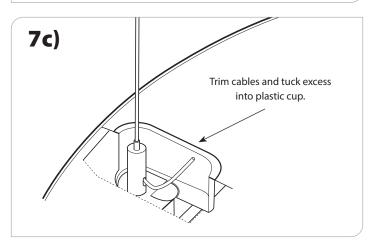
Field cut SJT cord to proper length and strip back portion of outer insulation. Perform wire makeups above fixture (see color diagram below) and press wire nuts (by others) individually through %" hole. Use plastic strain relief provided to secure cord in place.
