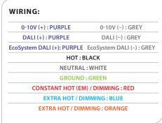
WARNING: Ground fixture in accordance with local and national electrical codes. Failure to do so may result in serious personal injury.
