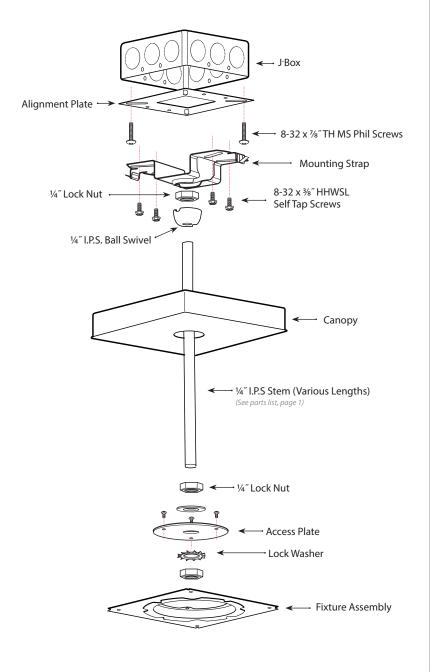
WARNING: Ground fixture in accordance with local and national electrical codes. Failure to do so may result in serious personal injury.
