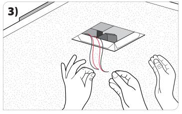
Disconnect AC wires and replace driver.
