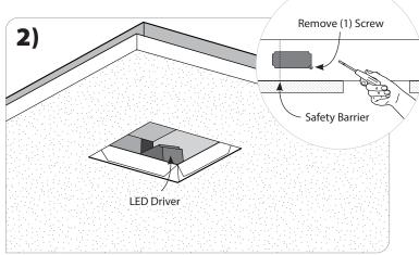
Remove (1) screw holding driver in place and pull driver away from safety
