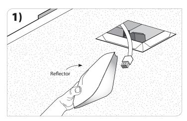
Remove reflector by pressing up and over to gain access. **NOTE:** The reflector is made of flexible plastic for easy removal.
