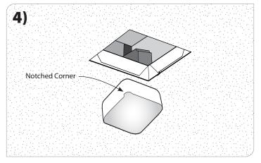
When reinstalling the reflector, note the notched corner is to be placed over DC LED wires where connected to LED boards.
