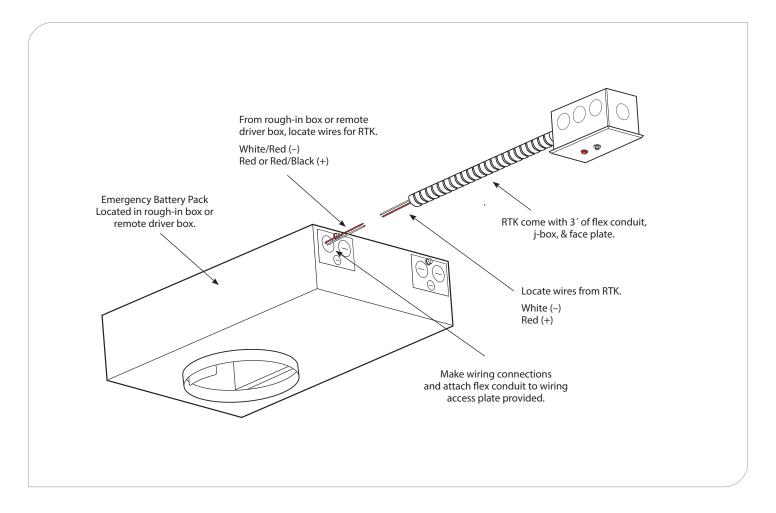
This product must be installed in accordance with the applicable installation code by a person familiar with the construction and operation of the product and hazards involved.
