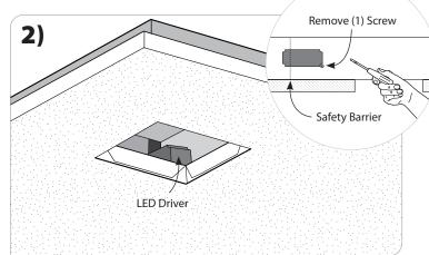
4. Unscrew driver from box, and remove to expose power disconnect
