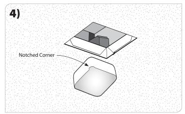
When reinstalling the reflector, note the notched corner is to be placed over DC LED wires where connected to LED boards.
