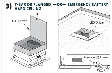
Replace driver from housing or locate in rough-in box. (AC building wire behind barrier)
