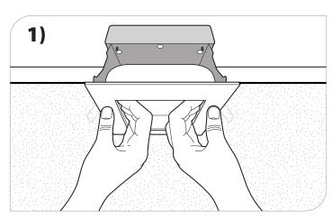
Remove fixture from ceiling by pulling from inside edge.
