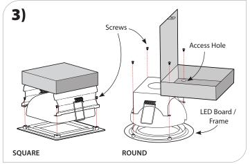
Remove (4) screws to detach trim frame. Unplug connector and remove LED board (note orientation of installed LED board). Install new LED board on trim frame and plug the connector. Attach trim frame using the same (4) screws.
