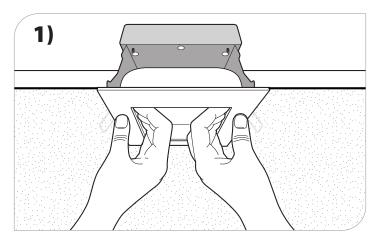
Remove fixture from ceiling by pulling from inside edge.
