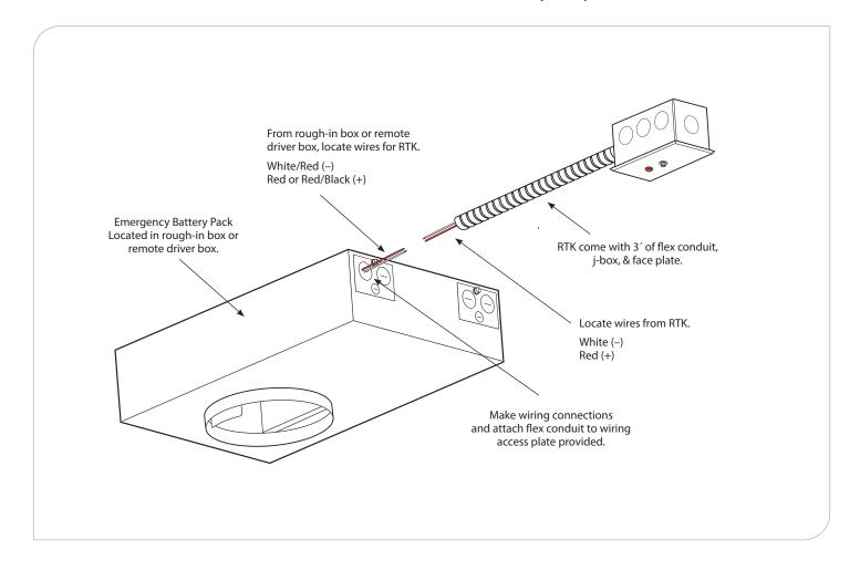
**WARNING:** Ground fixture in accordance with local and national electrical codes. Failure to do so may result in serious personal injury.
