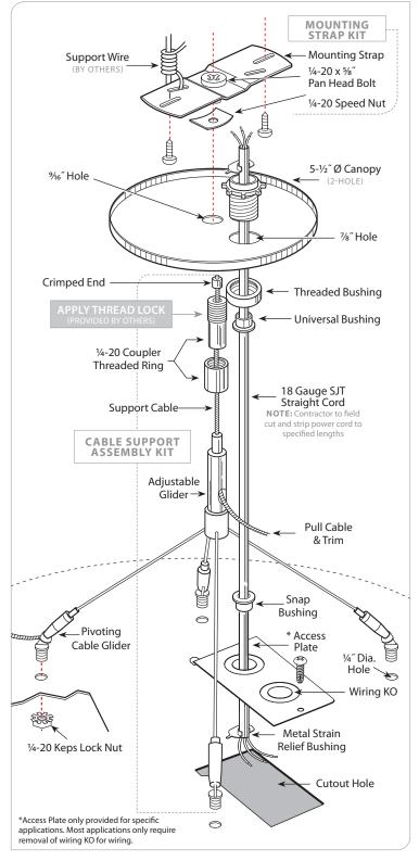
WARNING: Ground fixture in accordance with local and national electrical codes. Failure to do so may result in serious personal injury.
