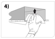
Push reflector into housing to proper position. Make sure no LED emitters are covered. Wire leads may need to be tucked away from emitters and reflector.
