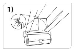
Hang reflector roll from same end using hook. **MATTE SIDE OF FILM WILL FACE DOWN** towards room when installed. (*Skip this step* on rows of 8' or less)
