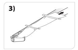
USE GLOVES PROVIDED. Pull reflector over entirety of housing row. Tighten roll to remove excess slack. Clamp roll to keep from unrolling.
