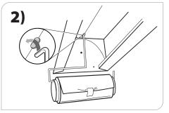
Hang reflector roll from same end using hook. **MATTE SIDE OF FILM WILL FACE DOWN** towards room when installed. (Skip this step on rows of 8' or less)
