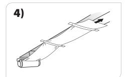
**USE GLOVES PROVIDED.** Pull reflector over entirety of housing row. Tighten roll to remove excess slack. Clamp roll to keep from unrolling.
