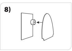
Install finish end plate to magnets on each end of row. Adjust end plate as needed to close gaps along reflector.
