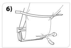
Cut reflector to fit — from side with excess reflector (hook & roll side). **DO NOT UNDER-CUT.** Make small cuts until reflector fits into housing, covering curved end plate.
