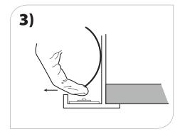
Use gloves provided. Gently lift bottom edge of reflector and remove from housing.
