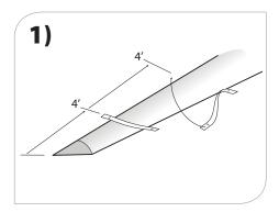
Locate faulty LED Rail or Driver. Starting at nearest end of row, attached tape strips approx 4' beyond faulty equipment.
