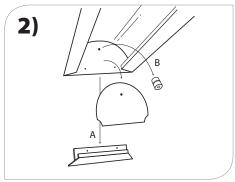
Remove end plate, magnet and end trim (when possible).
