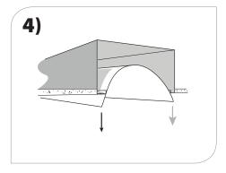
**USE GLOVES PROVIDED.** Pull reflector over entirety of housing row. Tighten roll to remove excess slack. Clamp roll to keep from unrolling.
