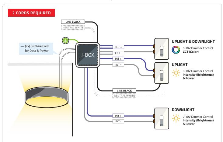
— Cords (Power and Data) between fixture and junction box are supplied by Prudential, but ship separately. Wire colors shown below are representative of the wires inside the fixture.
