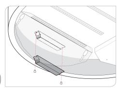
Disconnect LED modules wires from electrical wires. Remove screws holding driver in place. Rotate and lift driver out of fixture using quick connectors.
