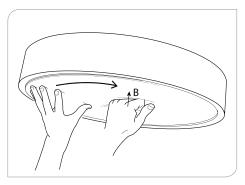
3. Press lens down in middle with one hand while pushing lens in along edge with other
