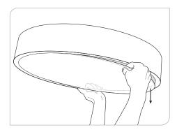
3. When more than 50% of lens is released (below trim), grab with both hands, flex lens in middle and remove
