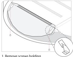
Remove screws holding reflector in place.
