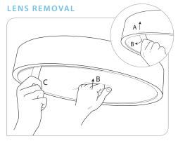
1. Insert lens removal tool (A), push lens up in middle of fixture (B) and pull back to pop edge of lens out
