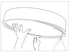
2. Slide tool slowly around rim to release lens (like a can opener)
